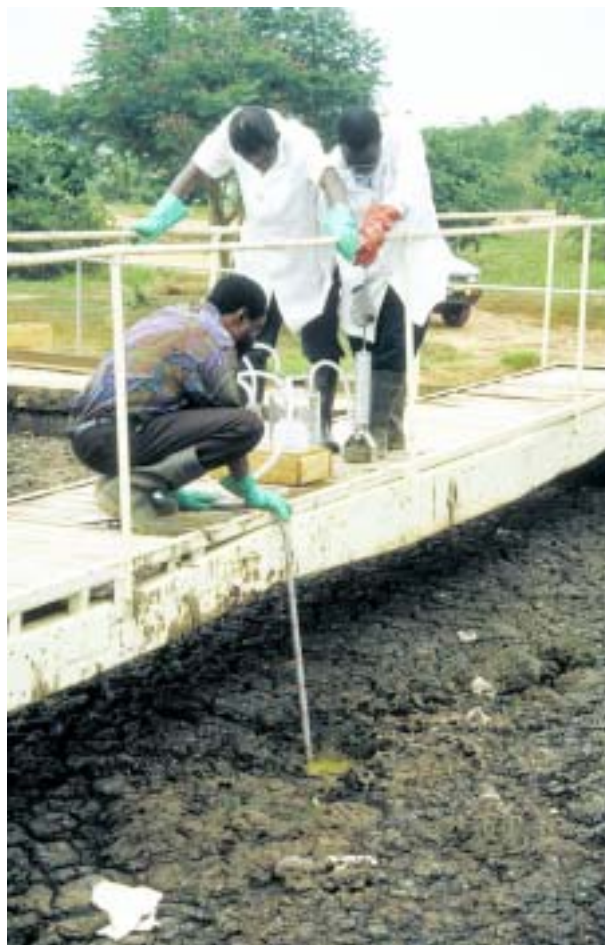
Figure 9: Learning from existing facilities and pilot plants: Sampling from a settling tank in Accra, Ghana
