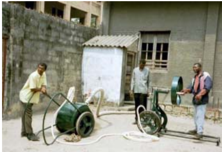
Figure 14: Small sludge tank connected to a hand-driven vacuum pump in Mapet, Congo.
