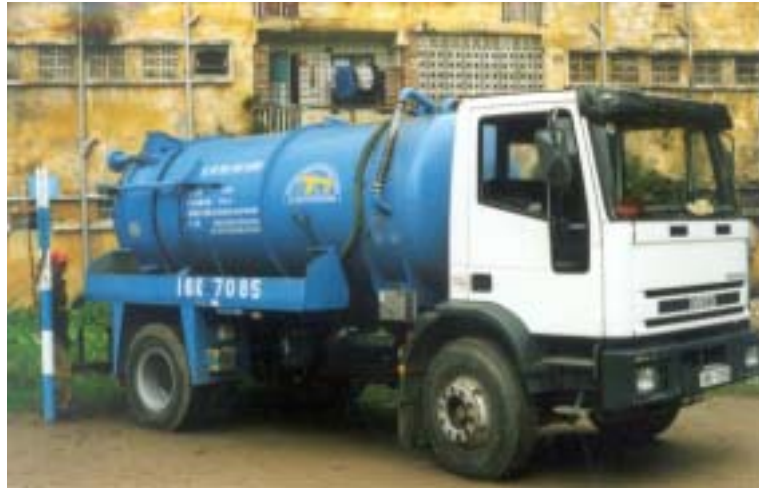
Figure 12: Truck mounted sludge tank (7,5 m 3 ) and vacuum pump in Hai Phong, Vietnam.
